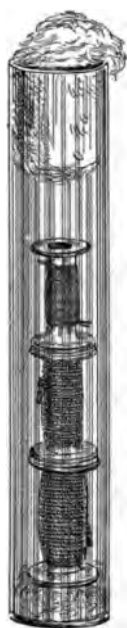
Fig. 156.—Silk in glass tube on glass reels; the tube is stoppered with cotton. (Hirst.)
